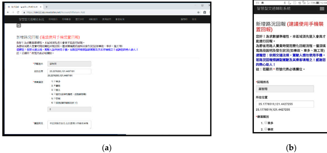
Figure 14. Road condition user reporting function displays for a (a) computer and (b) mobile phone. After logging into the system, when a user arrives at an accident emergency site, their intelligent handheld device can read the longitude and latitude of their location through the built-in GPS function, and present it in real time on the reporting page to complete add road condition reporting information.
