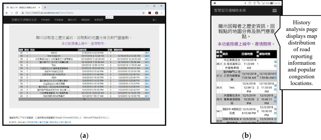
Figure 15. History analysis page displays map distribution of road reporting information and popular congestion locations for a (a) computer and (b) mobile phone. History analysis page of the system will obtain the return information through the cloud database; that is, clicking on the navigation function of the page will open the icon of the Google Maps display endpoint and go there.
